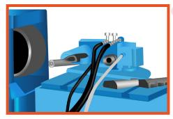
Rotary fixture on Rise & Fall Table. The casting is moved into position then rotated up to 108 degrees removing the risers. This picture shows a finished and unfinished part side by side.
