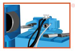
Rotary fixture on Rise & Fall Table. The casting is moved into position then rotated up to 108 degrees removing the risers. This picture shows a finished and unfinished part side by side.
